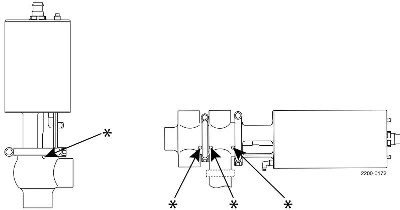
\* = Leakage detection hole
