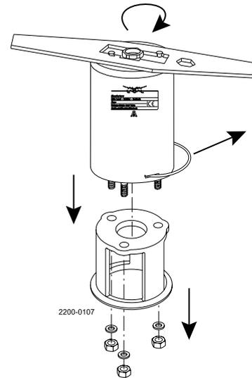
**Note!** The A/A actuator has no spring assembly.
