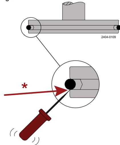
\* = it is important to place the screwdriver underneath the plug
