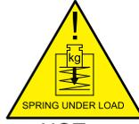
Do **NOT** attempt to cut the actuator open due to spring under load danger!
