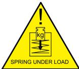
If marked with this warning, do **NOT** attempt to cut the actuator open, due to spring under load danger!
