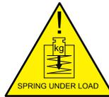
If marked with this warning, do **NOT** attempt to cut the actuator open, due to spring under load danger!
