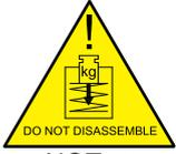
Do **NOT** attempt to disassemble the actuator due to spring under load danger!
