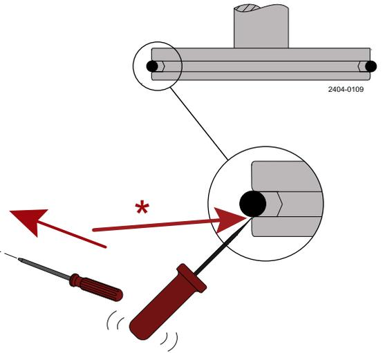
\* = It is important to place the screwdriver underneath the plug.
