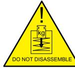
Do **NOT** attempt to disassemble the actuator due to spring under load danger!
