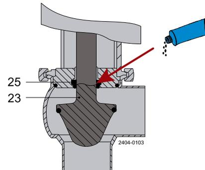
**Step 5****Lubrication of actuator**
