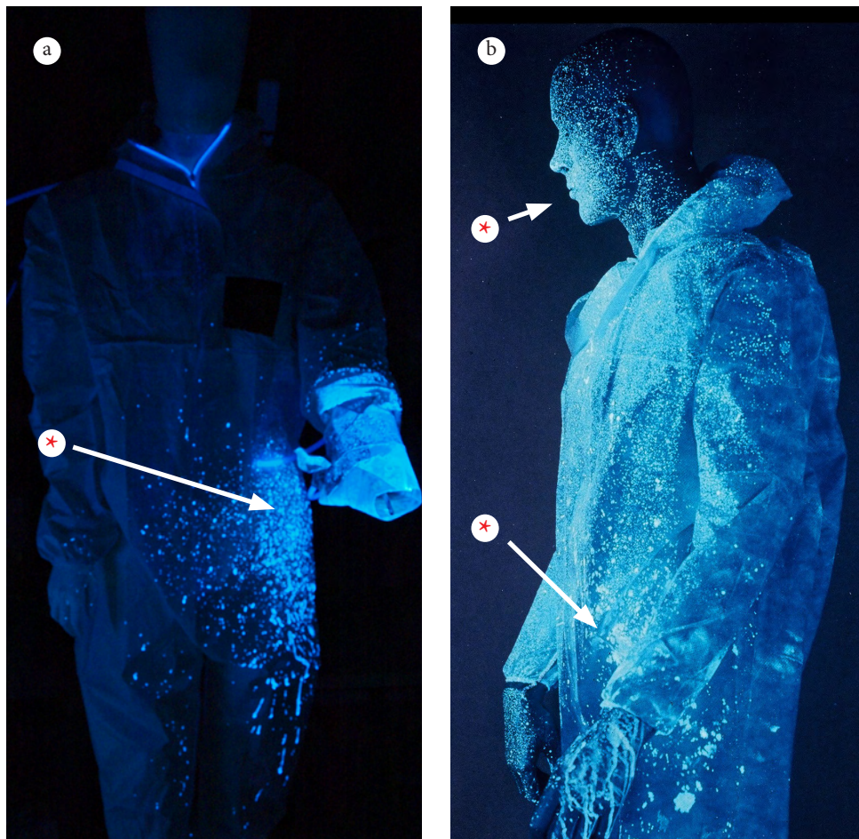
Figure 17: a and b) Photographs of MWF contamination on the torso and face (of a manikin) showing the effects of using a compressed airline and splash back onto the operator (The asterisk marks the spots / deposits on the face and arm visualised by adding a fluorescent blue dye to the MWF c
