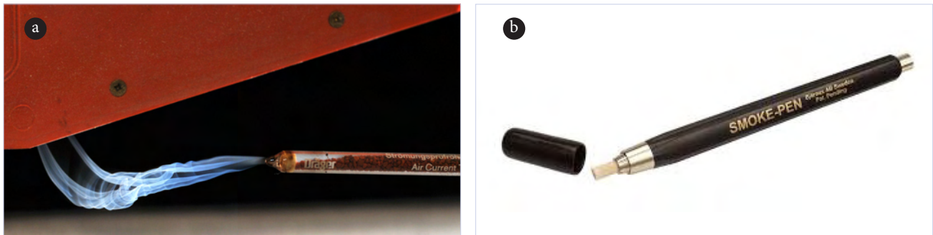
Figure 15: a) Shows a smoke tube, b) a smoke pen. These devices can be used to visualise any leakages in the equipment. Leakages would be detected by the release of smoke around the seals of equipment using back-lighting
