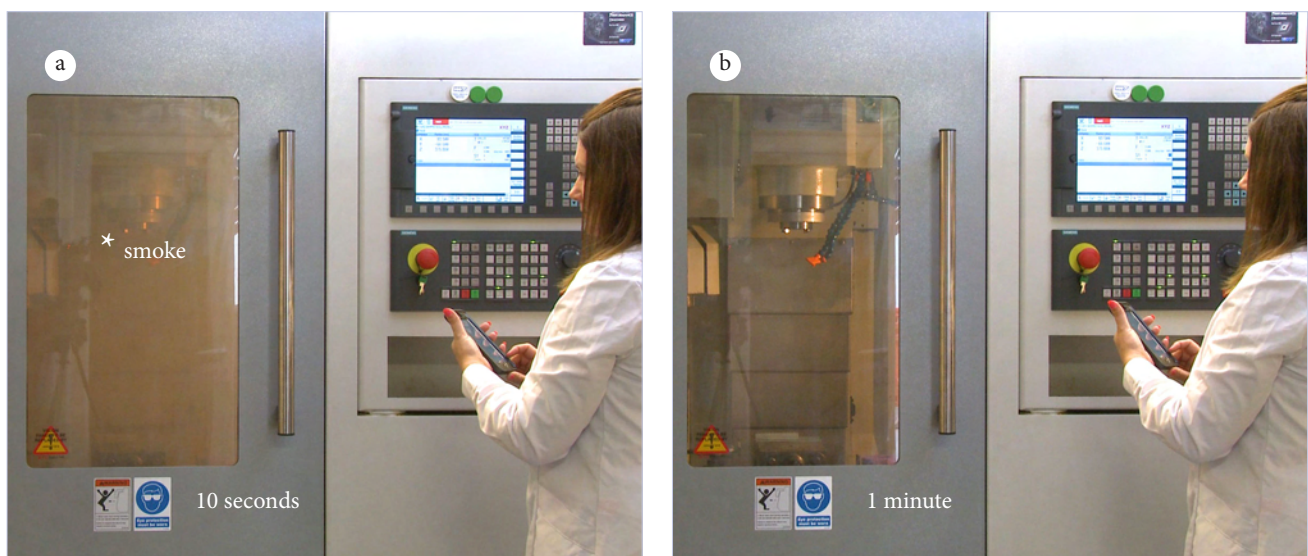
Figure 16: a) Back-lit photograph of smoke generated inside a machine enclosure after 10 seconds, b) shows clearance of the smoke within a minute. Note, this is an example of a clearance time, which may differ under other circumstances.
