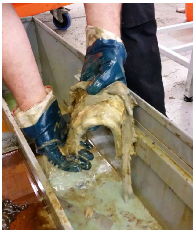
Figure 5: Biofilm deposits on the inside of MWF supply trunk.
